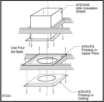
Fig. 33 Install firestops and attic insulation shield.
